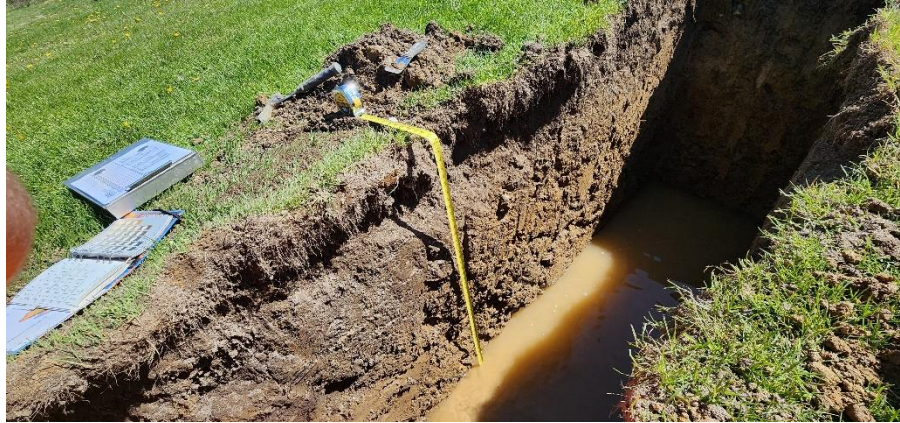
Photo #3 – TP-102 – Note High Groundwater Limiting Horizon
