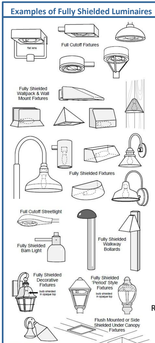
Figure 2. Examples of Fully Shielded Luminaires.
